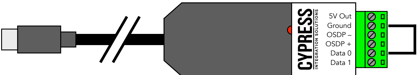
Figure 2: WDG-6112 Test Mode wiring
