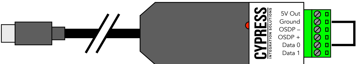
Figure 2: WDG-6112 Test Mode wiring
