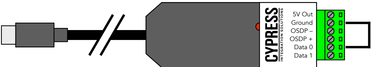
Figure 2: WDG-6112 Test Mode wiring
