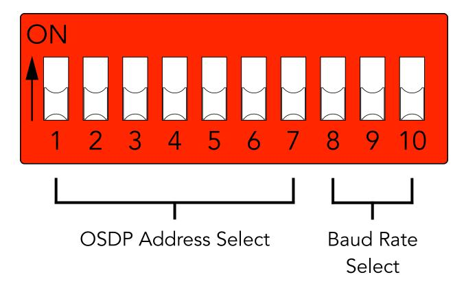
The OTT-2100 has a 10 position DIP switch bank that is used to select the OSDP address and the baud rate that the OTT-2100 will configure in the connected OSDP reader or PD. The DIP switch is ON when the switch is pushed away from the number on the DIP switch bank, or towards the 2-pin header/connector. The DIP switch is OFF when the switch is pushed toward the number on the DIP switch bank, or towards the Status LEDs.
