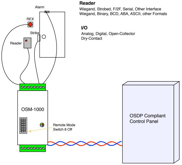
Power for the OSM-1000 can be supplied by the panel on a separate pair or be supplied locally at the door.
