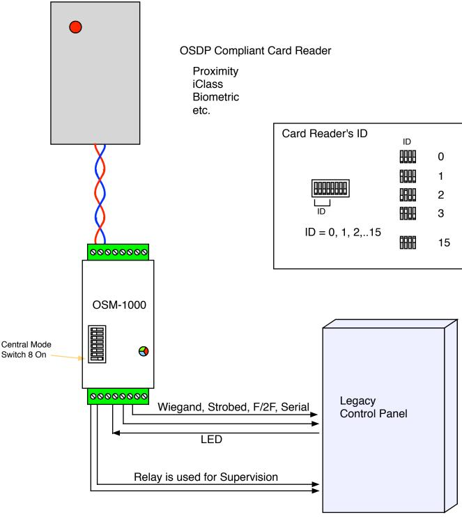
If Secure Channel is used (Sw 7 On), the OSM-1000 will initiate the authentication sequence with the device whose polling ID matches the DIP switch setting (or configured via OSDP *COMSET* command).
