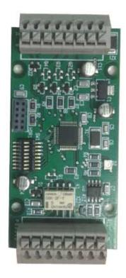
The OSM-1000 is the first in a family of products that are specifically designed to allow legacy card access panels and readers to interface with the SIA - Open Supervised Device Protocol (OSDP). Wiegand, Serial, Strobed, ABA, Bar Code, and other widely used interfaces and formats are re-packaged into an equivalent OSDP packet structure. The OSM-1000 can be field configured to be a reader-side (PD) or panel-side device (CP).
